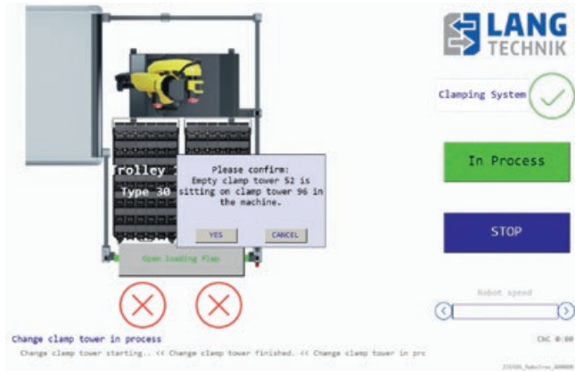
Figure 38: Replacing the zero point clamping system
