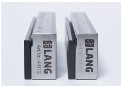
Left: Stamping jaw with original thickness of 18 mm. Right: Reconditioned stamping jaw with a thickness of 15 mm.
