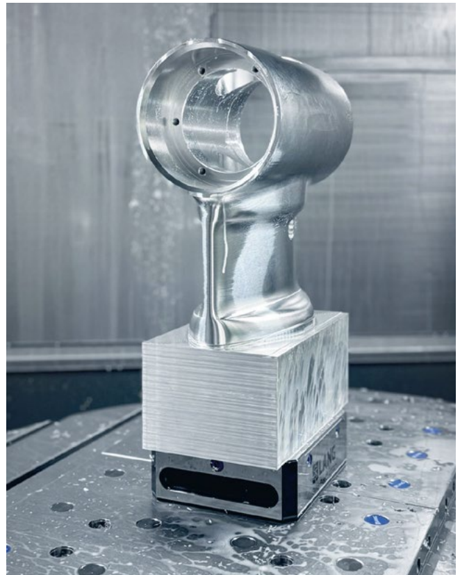
Direct clamping of a gearbox via four clamping studs with over 80% material removal.
