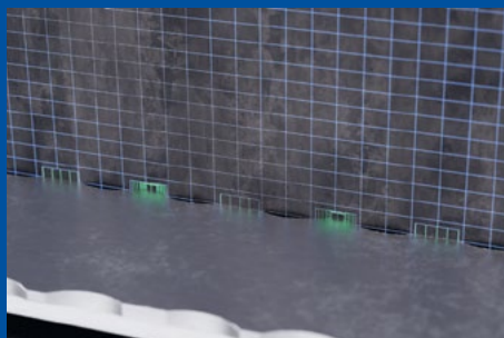
Form-fit clamping of pre-stamped blanks with Makro·Grip® serration
