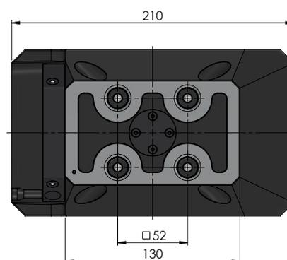
**AUTOMATION-NULLPUNKTSPANNSYSTEM 52, PNEUMATISCH**
