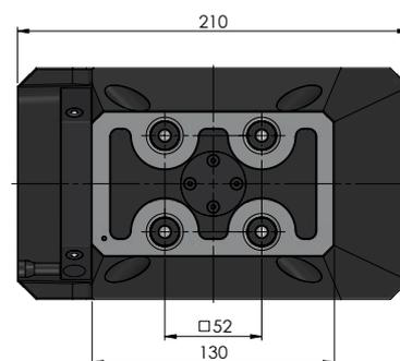
AUTOMATION-NULLPUNKTSPANNSYSTEM 52, PNEUMATISCH
