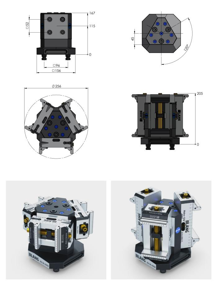
With horizontal mounting, three Makro-Grip® 77 5-Axis Vises with a maximum length of 130 mm can be clamped in the Tri-Top (left). Clamped vertically, a maximum vise length of 170 mm is possible (right). Shorter lengths and smaller sizes can of course also be used.
