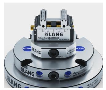
From big to very small – Even with the Quick•Point<sup>®</sup> 96 zero point clamping system, the Makro•Grip<sup>®</sup> micro can be used. This is made possible by additional adapter plates, which also provide extra accessibility in 5-sided machining.
