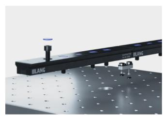
Extension bars can be added to the left and right of a clamping bar. A continuous 4 mm grid is created across both bars, which allows the risers to be moved flexibly.
