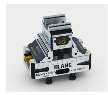
The micro vise has a hardened stamping contour in the base body, which allows it to be clamped in any Makro-Grip® 77 and 125 with high positioning accuracy. It thus offers a flexible option for quickly machining small components on 5 sides with large and medium-sized vises.
