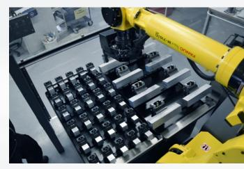
RoboTrex 96 with gripper exchange interface and different sizes of trolleys. Image: Waibel GmbH CNC-Teilefertigung
