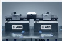
In order to provide an additional resting surface, a support jaw can be mounted.
