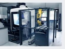
RoboTrex 52 retrofitted to a DMU 50 by DMG Mori.
