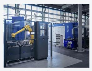
2 Grob G350 machine tools with RoboTrex 96 and 52. Image: Lindauer DORNIER GmbH
