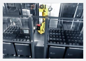
4-trolley RoboTrex 52 version attached to a DMU 60evo. Image: Peter Josef Klein Feinmechanik GmbH
