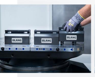
Adding further bases for an increased clamping range
