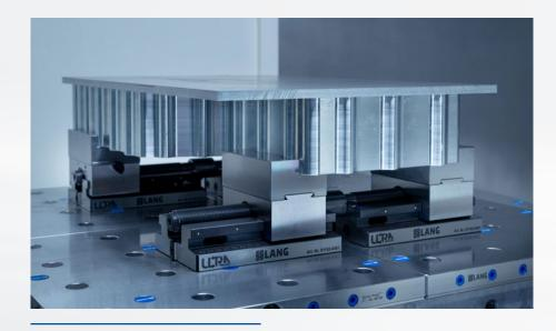
2nd OP / rear-face machining using contour jaws.
